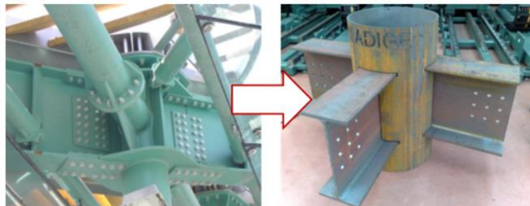
Figure 1.1: LASTEICON I-beam-to-CHS-column joint specimen (FELDMAN 2016).
