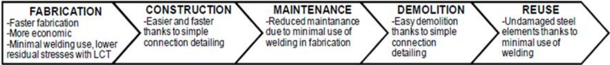
Figure 2.1: Scheme of the benefits of LASTEICON during the life cycle of a building project (CASTIGLIONI, et al. 2015).
